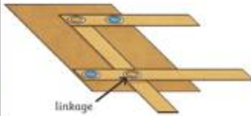
The part of the mechanism used to join one or more levers to produce the type of movement required.
