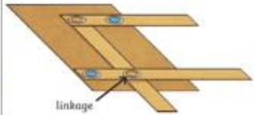
The part of the mechanism used to join one or more levers to produce the type of movement required.
